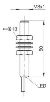
Inductive Sensors BES M08MI-NSC15B-BV02 M 8 x 50 normally-open Sn=1,5mm shielded
